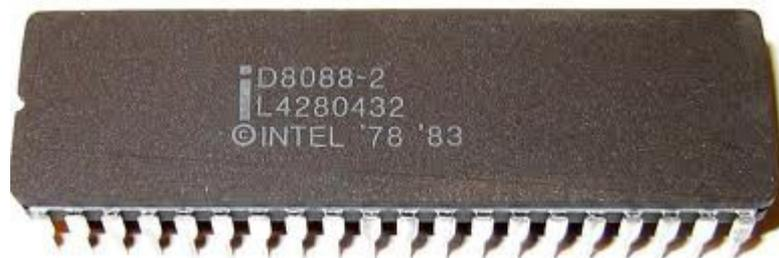
**Figura 24 – Processador IBM PC/XT.**
